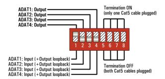
**ADX-64**: There are two DIP switch banks on the rear panel. Each bank sets the function for the corresponding 32 channel submodule.
