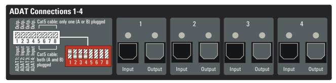
ADAT Lightpipe inputs and outputs 1-4. The transmission direction (transmit or receive) is set by DIP switches, see 7.1. Input/output mode (DIP switches 1-4).
